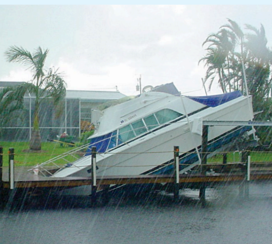
A boat on davits is extremely vulnerable to storm surge. If possible, store the boat ashore.
